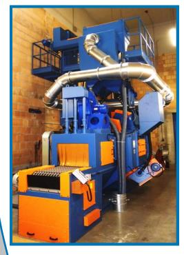
The closed and continuous circulation of the shot-blasting media is ensured by a screw conveyor, bucket elevator, abrasive cleaning air classifier unit and a feeding unit. In foundries an additional magnetic drum separator is built in the machine to separate forming sand from the circulation.
