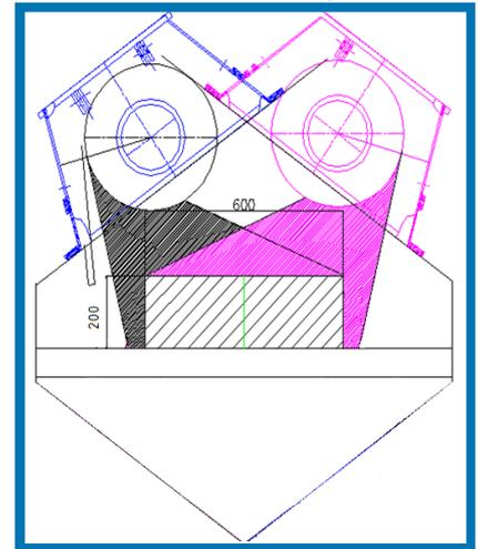
Due to the 2 blasting turbines on the top this machine provides fast cleaning speed for this cross section on one side.
