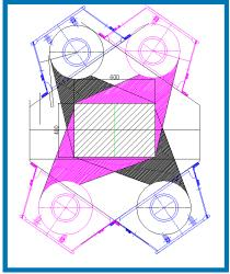
Due to the 4 blasting turbines this machine provides fast cleaning speed for this cross section.
