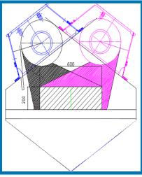
Due to the 2blasting turbines on the top this machine provides fast cleaning speed for this cross section on one side.
