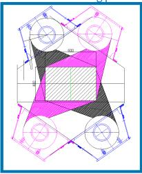
Due to the 4 blasting turbines this machine provides fast cleaning speed for this cross section.
