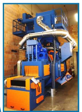
The closed and continuous circulation of the shot-blasting media is ensured by a screw conveyor, bucket elevator, abrasive cleaning air classifier unit and a feeding unit. In foundries an additional magnetic drum separator is built in the machine to separate forming sand from the circulation.
